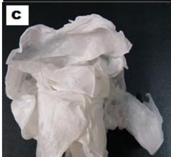
Fig 4b: Image of purified wet cellulose layer c Image of dried cellulose layer.
