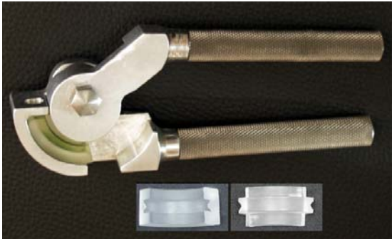
Fig 4: Home-made hand juice squeezer with changeable and sterilized plastic shells. 50–60 mg of the potato leaf tissue is cut into strips, placed in the cavity of left shell and then the right convex shell is set into the cavity. Both shells have terminal recesses that while combined form terminal wells. Combined shells are put into the squeezer and cell juice is pressed out into shell wells and picked up with a micropipette.
