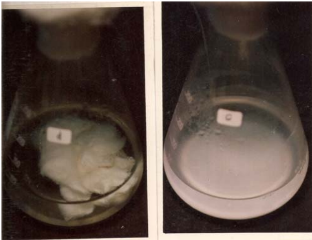
Fig 1: Adsorption of lead carbonate from distilled water by fresh biomass of Rhizopus sp. (d). Water containing lead carbonate, but lacking biomass (C).
